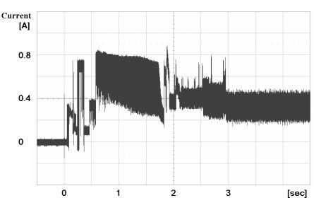
(6) Current fluctuation (Typ.) at +5 V when power is turned on
